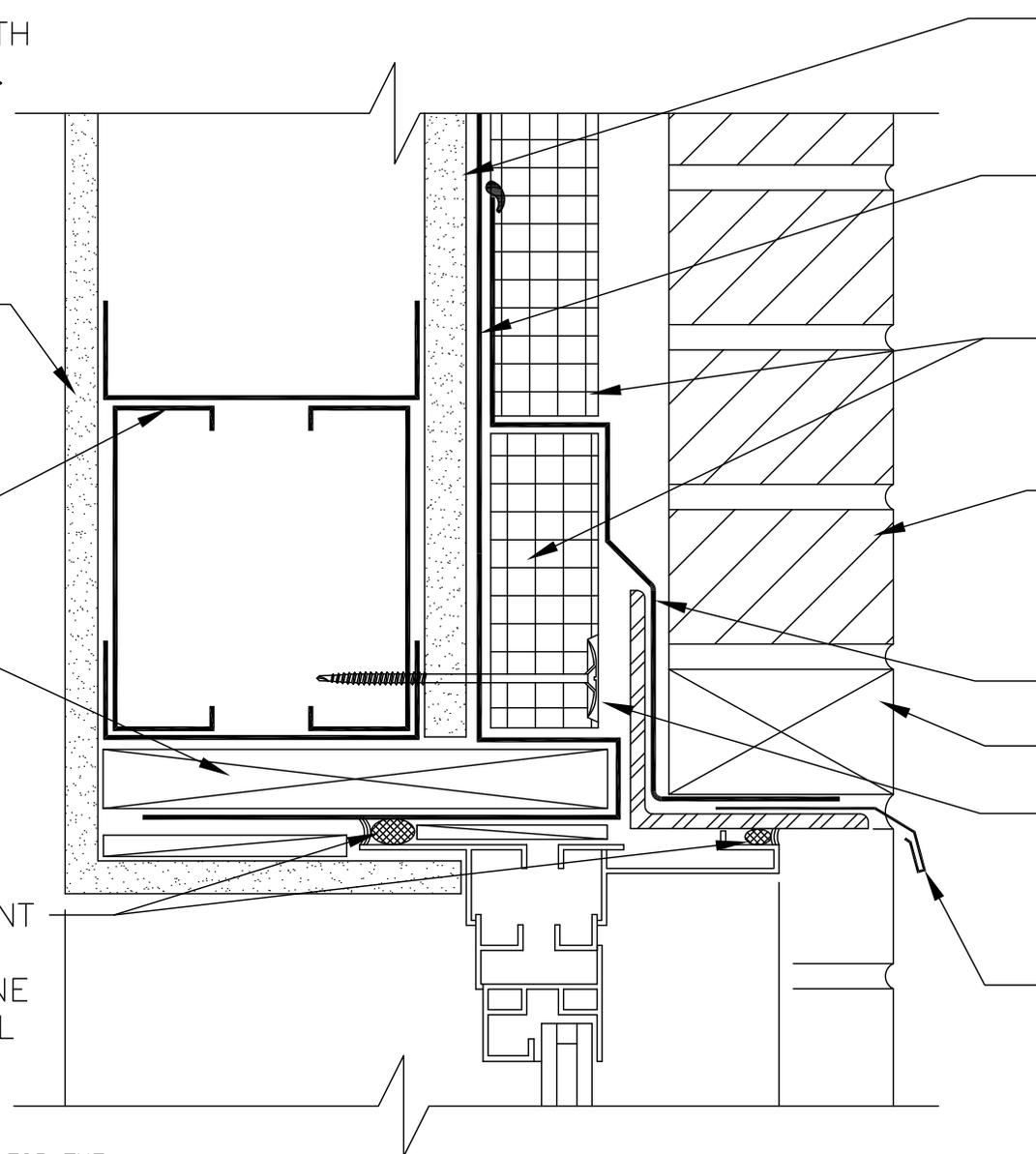
DETAIL IS INTENDED TO BE A GUIDE FOR THE INSTALLATION OF CCW PRODUCTS ONLY. DETAIL SHOWN IS SUITABLE FOR USE IN NFPA 285 WALL ASSEMBLIES. USE WALL ASSEMBLY COMPONENTS AS LISTED IN R2-0B, R2-0C AND R2-0D DETAILS.
