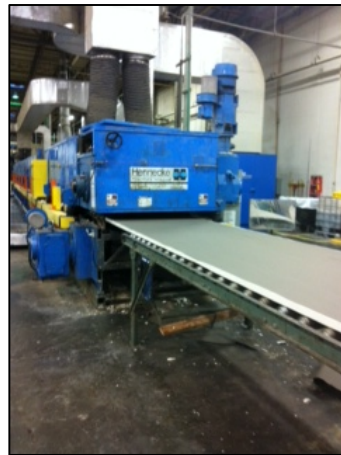
Resin expands and cures, filling space between facers
