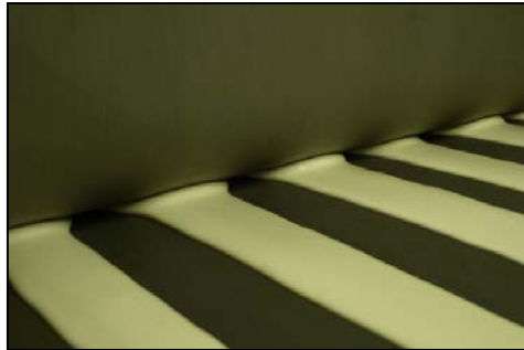
Beads of mixed 2-part resin extruded onto facer
